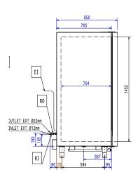
Drain Electrical inlet (power) RΩ Refrigerant Outlet
